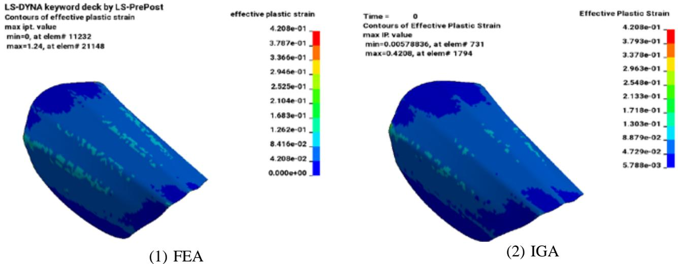
Figure 3: Effective plastic strains obtained via the one step approach using (1) FEA and (2) trimmed NURBS-based IGA.
