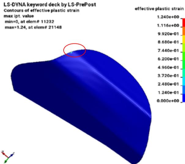
Figure 4: Localized effective plastic strain in the FEA model.
