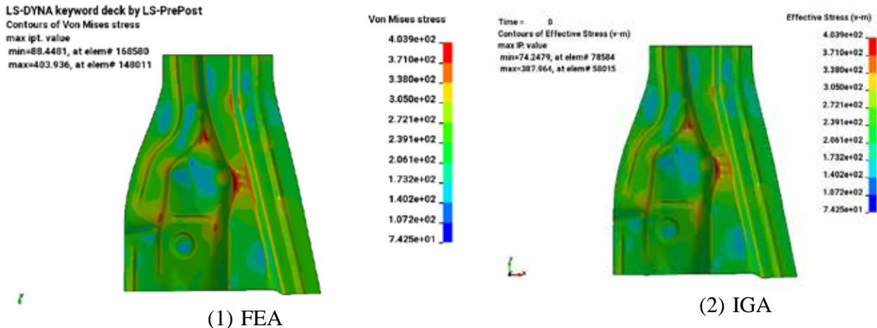
Figure 1: Von Mises stresses as a result of the one step analysis using (1) FEA and (2) untrimmed NURBS-based IGA
