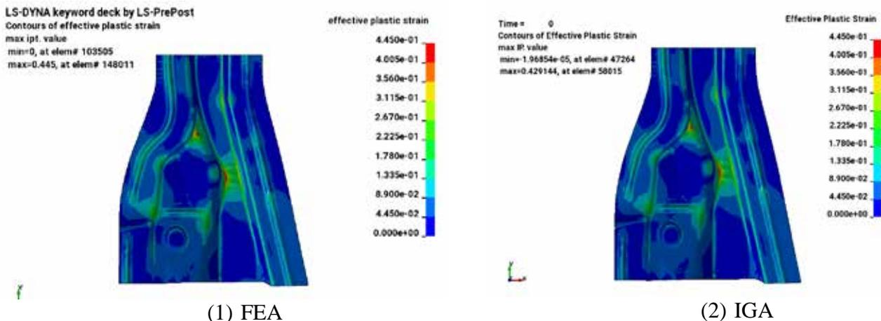
Figure 2: Effective plastic strains obtained via the one step approach using (1) FEA and (2) trimmed NURBS-based IGA.
